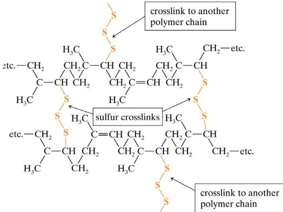
Natural rubber latex is made much more useful by adding crosslinks. (a) Two strands of polyisoprene (rubber). (b) Sulfur reacts by opening the double bonds in the polymer and forming bridges between adjacent strands. The product is called vulcanized rubber.
